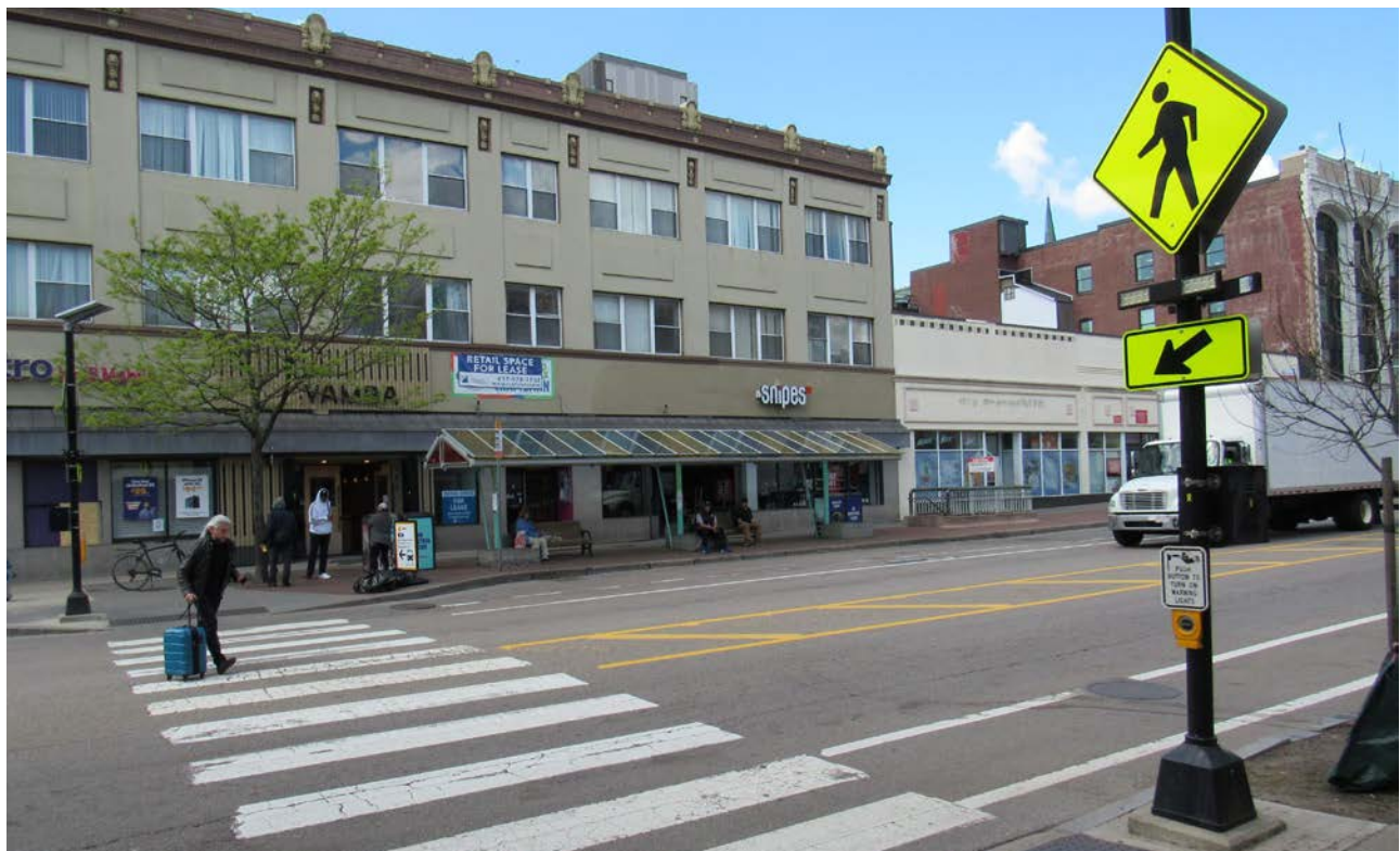
Figure 4-4: Rectangular Rapid Flashing Beacon in Central Square, Cambridge, MA
