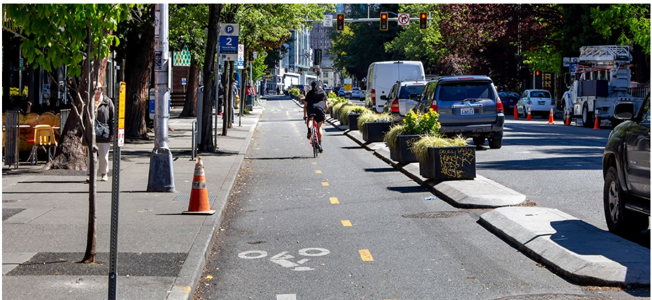
Figure 4-26: Roadway Reconfiguration with physical separation
